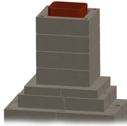
Figure 19. Masonry Chimney Assembly
