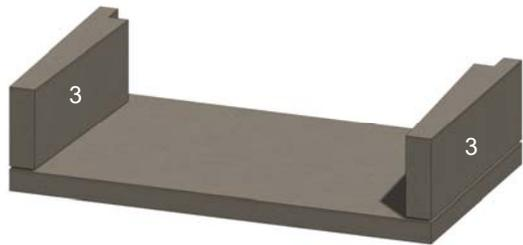
Figure 9. Lower Sidewalls
