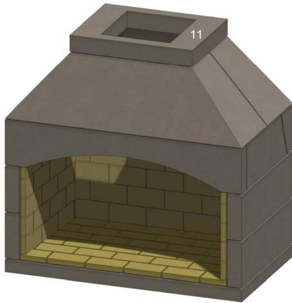
Figure 20. Flue Adapter
