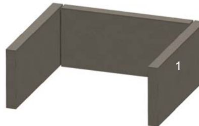
Figure 9. Riser Legs & Cross-Leg
