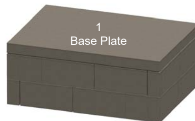
Figure 6. Kit Base Plate on Block Base
