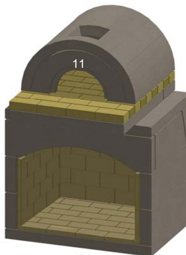
Figure 24. Oven Front Wall
