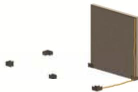
2. Begin at a corner, securing to the pad, and set the beads of adhesive for the adjoining end panel.
