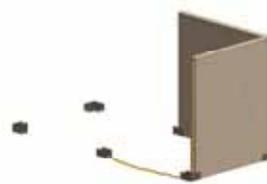
3. Add 1st end panel, securing to wall panel and adding adhesive beads for the bottom and end joints.
